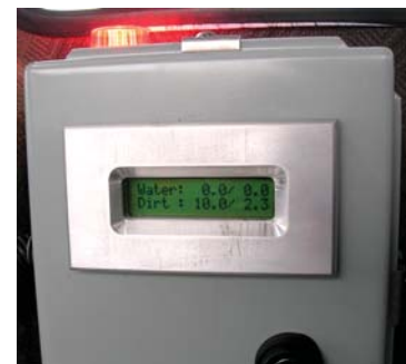
Modular readout of dirt (mg/l) and water (ppm) readings
